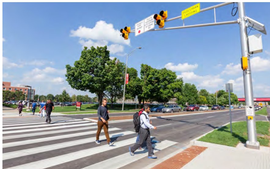
High Intensity Activated Crosswalk (HAWK) signals are a type of pedestrian activated crossing. Source: Indiana University
